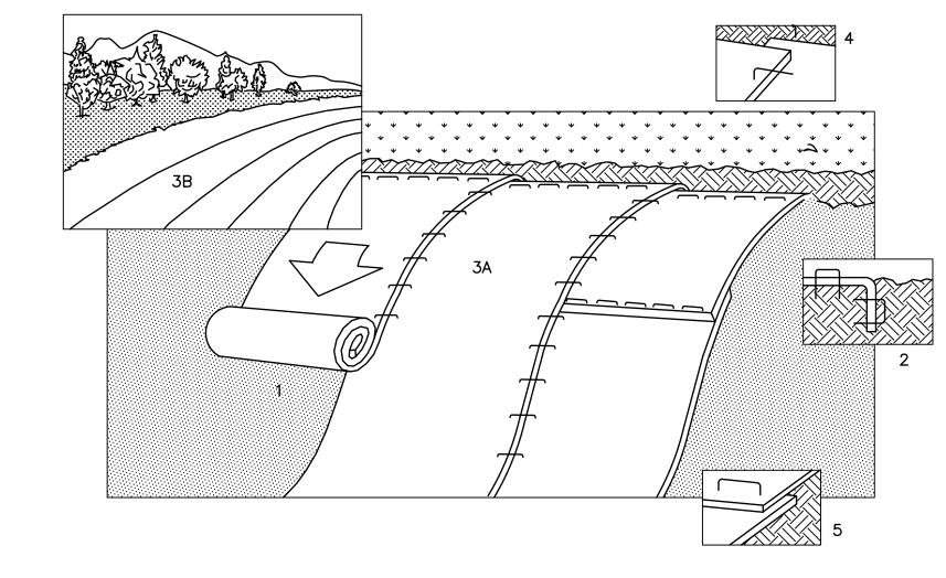
1. PREPARE SOIL BEFORE INSTALLING BLANKETS, INCLUDING APPLICATION OF LIME, FERTILIZER, AND SEED. 2. BEGIN AT THE TOP OF THE SLOPE BY ANCHORING THE BLANKET IN 6" DEEP X 6" WIDE TRENCH. BACKFILL AND COMPACT THE TRENCH AFTER STAPLING.
