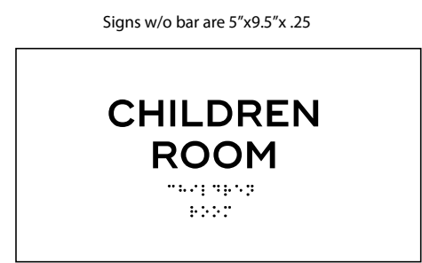
Elevation ADA Signage Showing Layouts W/O Bar Scale: 3" = 1'-0" ITEMS: See Message Schedule
