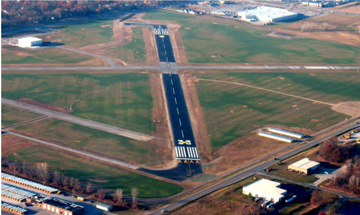
Figure 2-3. Markings for a Temporarily Closed Runway
