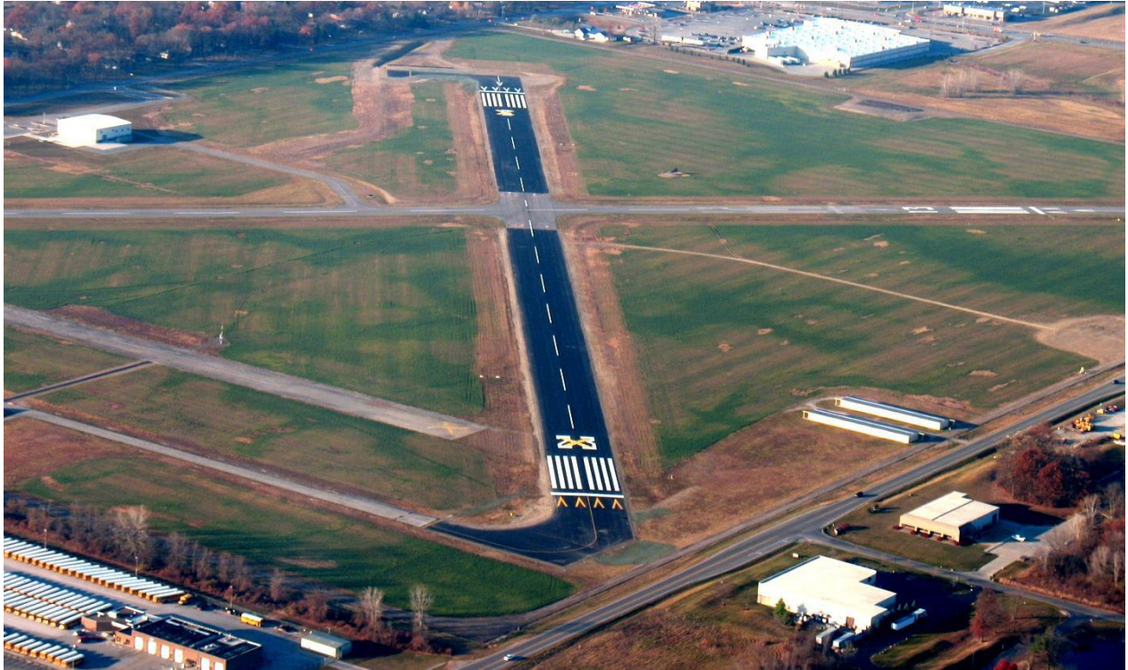
Figure 2-3. Markings for a Temporarily Closed Runway
