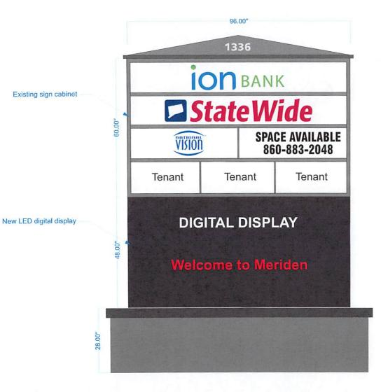
One 48" x 96" two sided cabinet with LED digital display on each side. The existing sign cabinet will be moved up and the new LED digital display will be located below the existing sign cabinet.
