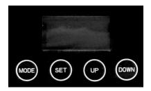
Operation Mode Transformation - press 'MODE', then 'UP' or 'DOWN' button to transform menus:
