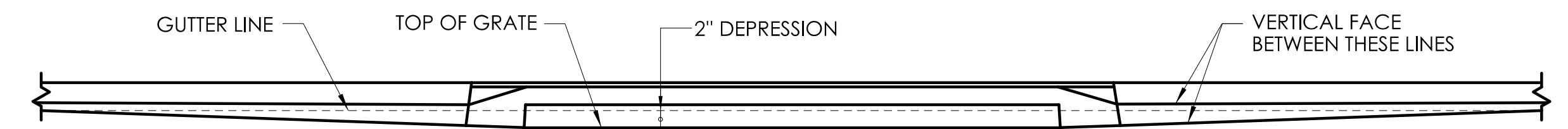
CATCH BASINS IN A LINE WITH 4" CONCRETE PARK CURBING OR 4" BITUMINOUS CONCRETE PARK CURBING
